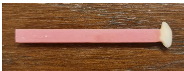
Figure No. 1: Specimen (denture base and acrylic tooth)
