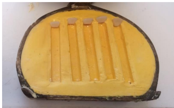
Figure No. 3: After dewaxing
