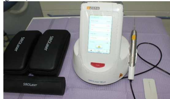
Figure No.1: SIROLaser Blue, emitting light at 445 nm and operating at 2 W
