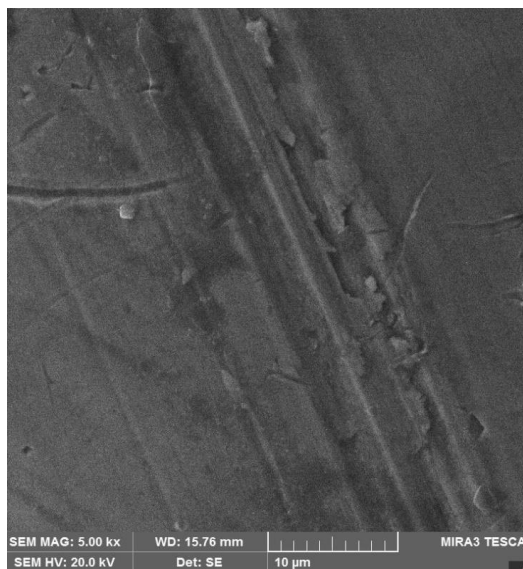
Figure No.2: SEM analysis of SS wire after potentiodynamic test in acid mouthwash
